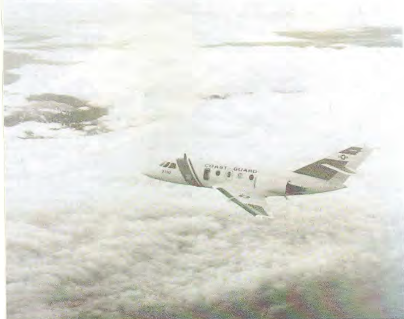
The HU-25A "Guardian", a new Coast Guard multi-mission jet, can operate from sea level to an altitude of 42,000 feet. Its 160-mile radius and five hour flight endurance make the Guardian a welcome addition to the Coast Guard's search and rescue and drug interdiction efforts.
