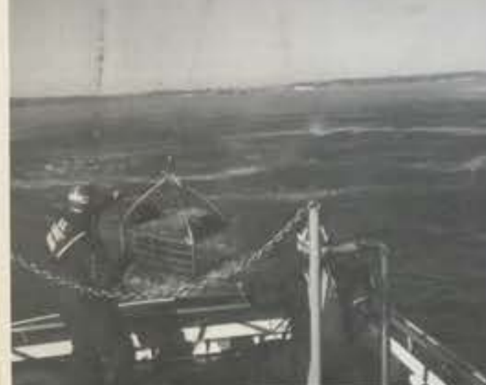
Crew members of Station Charlevoix's 41-footer use a trail line to bring the basket aboard. Meanwhile the helo has backed off so it is not directly overhead. When the helo is directly overhead, churning of the air column and water directly beneath it can create forces strong enough to turn a moderate-sized boat around unless the captain takes countermeasures to maintain his heading.
