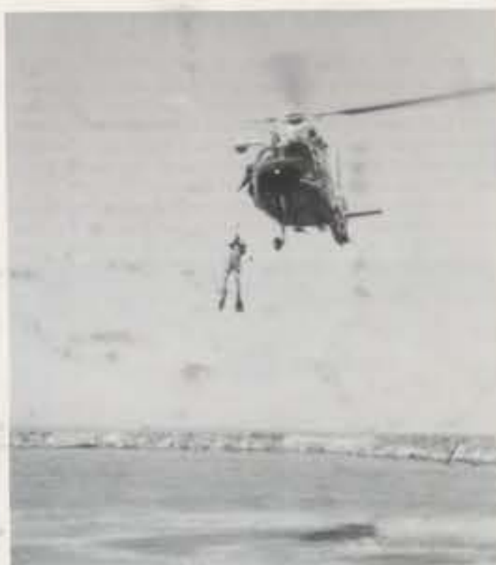
A rescue swimmer may be lowered to retrieve persons in the water. A swimmer may also be lowered when the helicopter crew cannot establish two-way comms with a vessel or when medical attention/stabilization is needed prior to a MEDEVAC hoist. Courtesy Ninth Coast Guard District.
