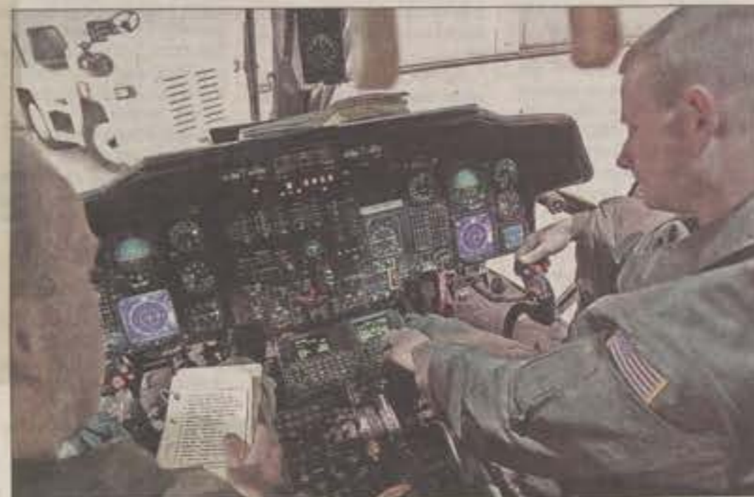
Lt. j.g. Gabe Somma and Lt. j.g. Jerod Glover practice going over the flight checklist. Pilots drill constantly to master the many different settings of 300-plus switches and dials. The HH-65A "Dolphin" helicopter is almost 100 percent digital.
