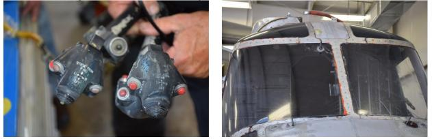
We inspected the horizontal sponson struts, which had been media-blasted and appeared to be in perfect condition and paint-ready. The Schrader valve atop the right main landing gear was free of corrosion and only needs layered paint removal. This update demonstrates that the 1426 restoration
