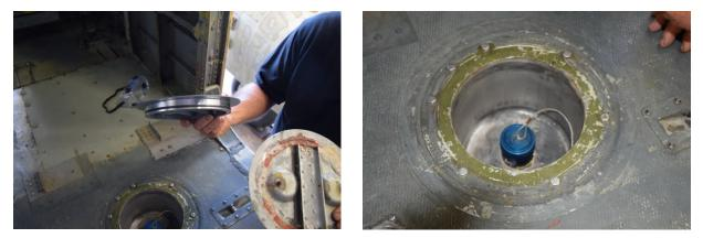
fuel tank access cover permitted Helicopter In-Flight Refueling (HIFR) by gravity feed nozzle from a WMEC or WHEC. You can easily see that the fitting in the HIFR well is in excellent condition. The
