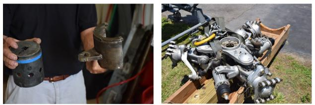
with a long steel bar to create 300 foot-pounds of torque) enabled VectorCSP to remove the rotor head from the splined transmission rotor shaft. Dampener boots and pitch change rod end covers will be inspected and renewed as necessary. "Tea kettle" hydraulic reservoirs will be drained. The "Jesus
