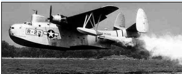
A CG PBM-5G, sister aircraft to #84738 that flew the Swatow mission, jet assisted take-off using JATO rockets. (CGAA)
