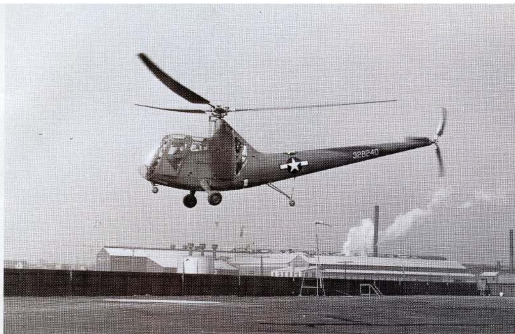
Twenty-seven Sikorsky HOS-1s were built by Nash-Kelvinator, an automobile and refrigerator manufacturer. Some of these aircraft were at the world's first helicopter school, Coast Guard Air Station Floyd Bennett Field, New York in 1944. Two crashed from in-flight failures with no fatalities. Igor I. Sikorsky Historical Archives
