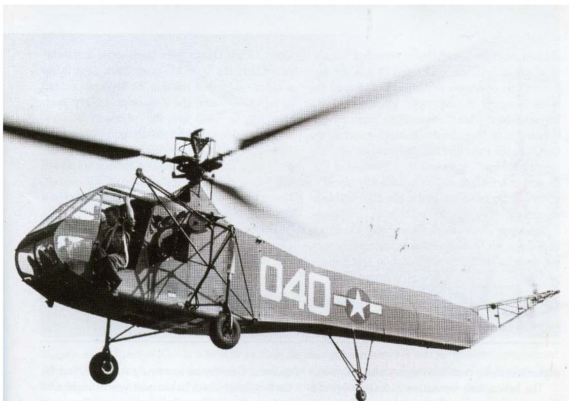
The steel-tube framed, fabric covered HNS-1 had wire-mesh stretched over the lower fuselage to make it a radar target for naval ships' guns calibration. The 200 horsepower engine was sometimes insufficient for flight on warm summer days, so the aircraft was lightened by removing the radio if two crewmen were necessary. This led to an unexpected and embarrassing first aircraft landing aboard the new aircraft carrier, USS Bennington (CV-20). Igor I. Sikorsky Historical Archives
